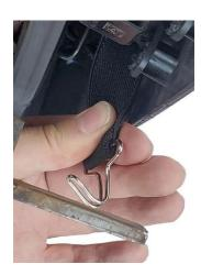
**Step 2C.** Attach the 2 front straps on pockets ("B" in photo) and the 2 side straps ("C" in photo) to springs on the underside of seat bottom (can also be secured to previously installed seat cover hooks). Side straps "C" are designed to go between the seat cushion and plastic molding leaving seat controls accessible, not over the plastic molding. If gap between cushion and plastic molding is too tight to insert strap, remove hooks from straps as detailed in step 2B.
