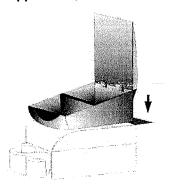
**Step 2.** Pass console bottom flap through opening, then attach velcro.
