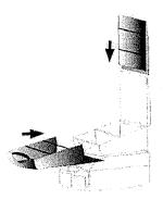
**Step 1.** Slide on console top, then console bottom.
