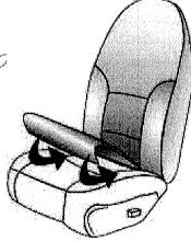
**STEP 2.** Pass the bottom flap through the opening between seat back and seat bottom, then attach velcro.
