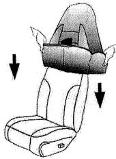
STEP 1. If the seat has an armrest, place it in the "up" position. If the cover has a zipper, unzip it. Pull cover over top of the seat. It may be helpful to start with the cover inside-out (as shown).
