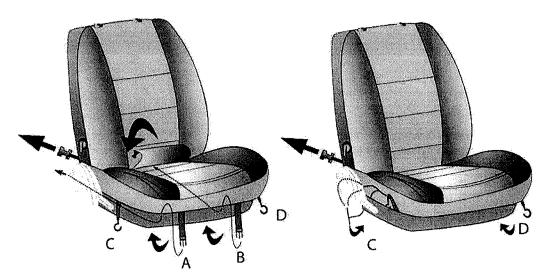
**Step 1.** Position cover over seat bottom. Pass flap between seat back and seat bottom. (Similar to the seat back cover installation, it may be easier if you fold the seat back forward) Join and tighten the buckles (A,B) under the seat.
